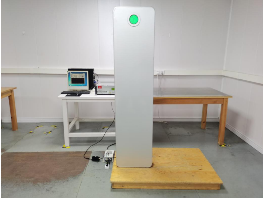
Photo of Injected Currents Susceptibility Test
