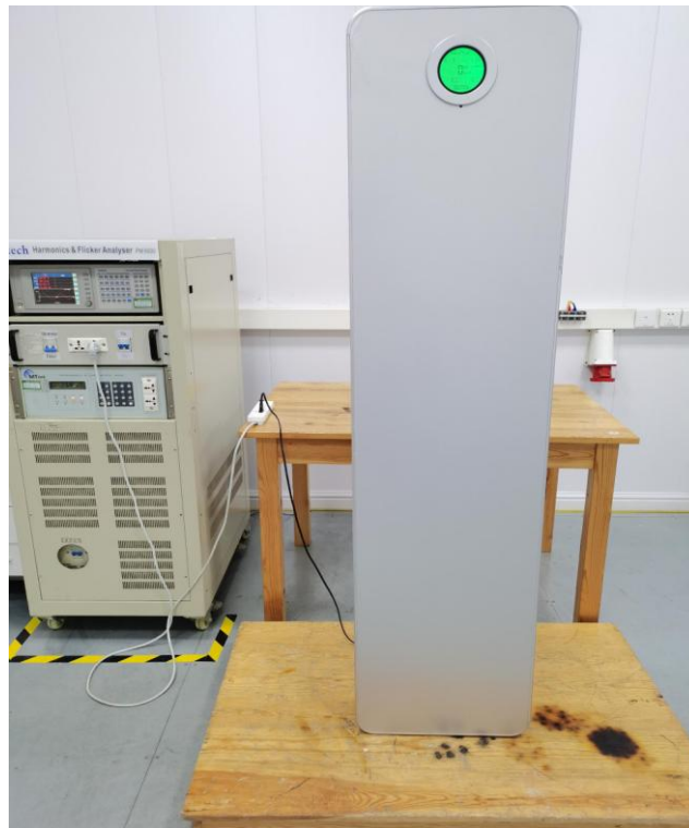
Photo of Harmonic & Flicker Measurement
