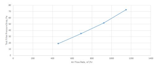
Resistance to Airflow (Loaded Filter, ISO 16890 part 3)
